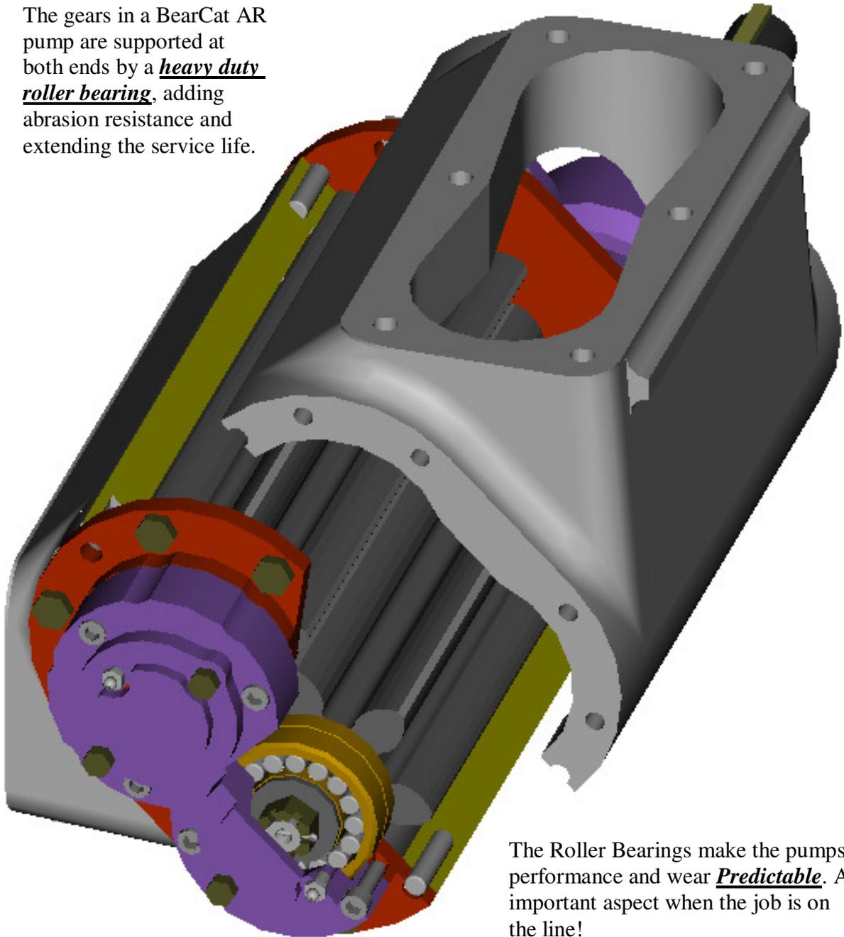
The Roller Bearings make the pumps performance and wear **Predictable**. An important aspect when the job is on the line!
